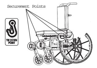
FIGURE 1 - SECUREMENT POINTS
